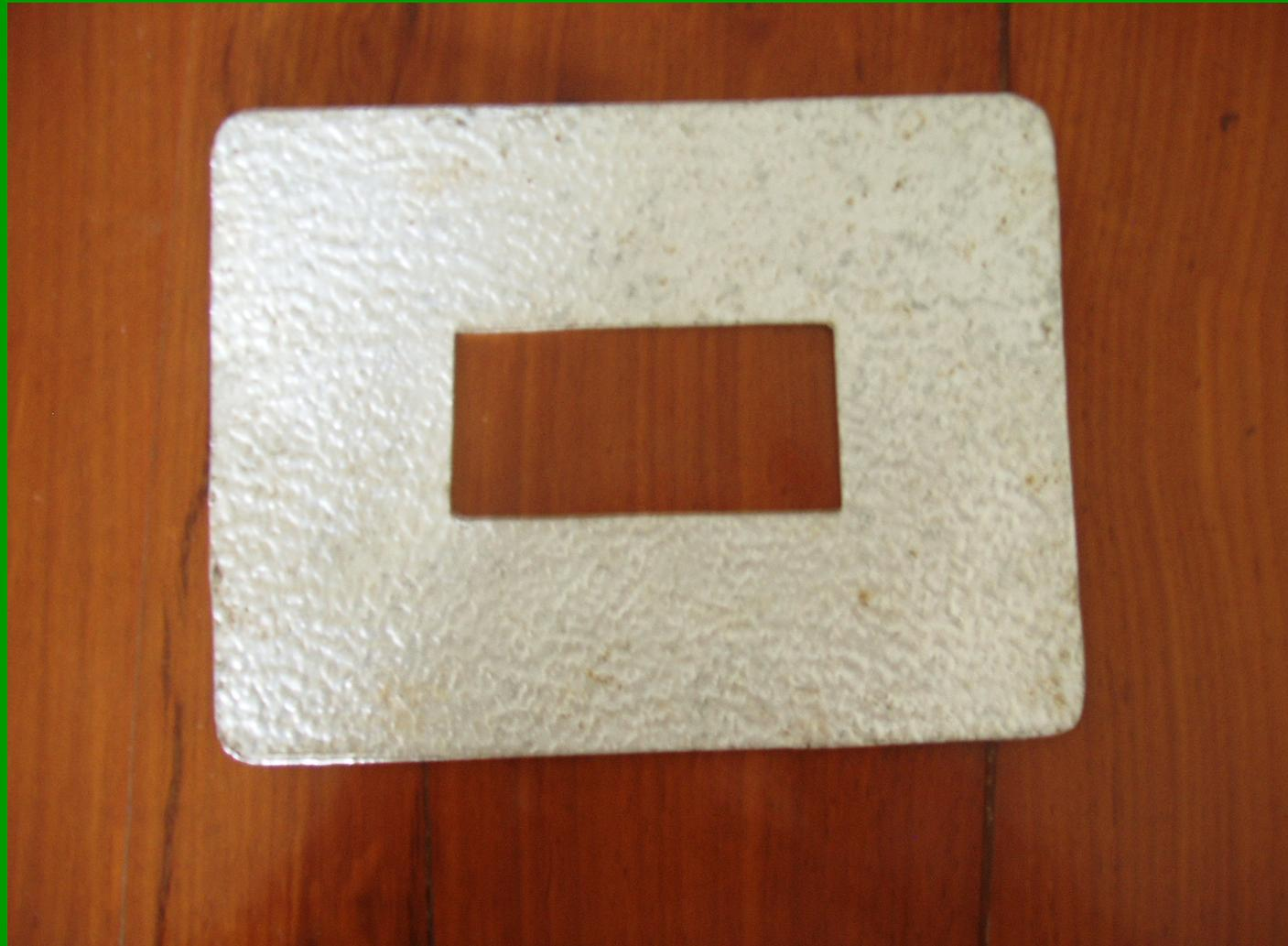
**Introduce a pin on each of the four internal corners to delineate the test area, and to be able to return and place the plate over the exact same area after 24-48 hours.**
