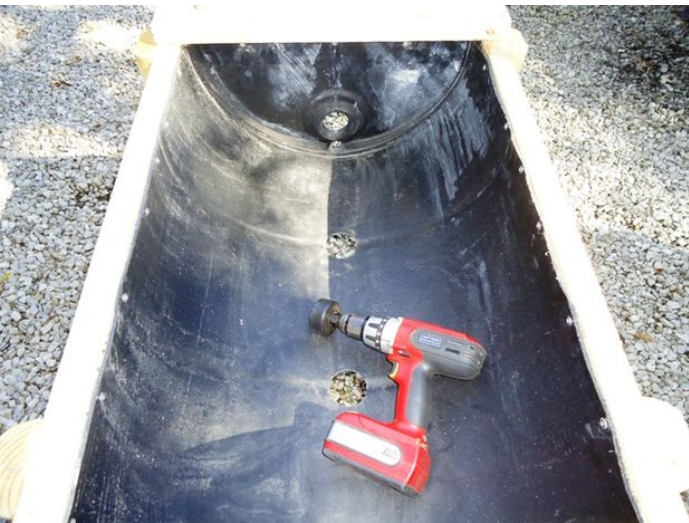
Step 49: Holes drilled and ready for screen.
