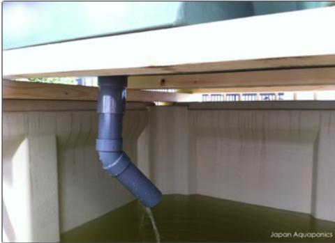
So you should now have the upper half of the Bell Siphon set up – the Bulkhead, The Standpipe, The Bell Siphon and the Media Guard. We can now look at the lower half of the Bell Siphon – the part that goes under the growbed.
